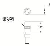
**Cartridge Style Visual Indicator** 3000 psi max Operating Pressure (6000 psi for 80 psid units) Temperatures up to 200°F **Automatic Resetting** Factory Installed. Available as kit for field replacement.
