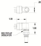
Cartridge Style Visual/Electrical Indicator DIN 43650 Type A Male Plug (11mm) 1NO, 1NC, & Common SPDT Switch (3 pole & ground) 5A; 125/250 VAC, 24 VDC (Resistive) 3000 psi max Operating Pressure (6000 psi for 80 psid units) Temperatures up to 200°F **Automatic Resetting** Factory Installed. Available as kit for field replacement.
