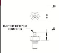
Cartridge Style Single Wire DC Indicator 200mA @ 36VDC Momentary - Normally Open Circuit 3000 psi max Operating Pressure (6000 psi for 80 psid units) Temperatures up to 200°F **Automatic Resetting** Factory Installed. Available as kit for field replacement.
