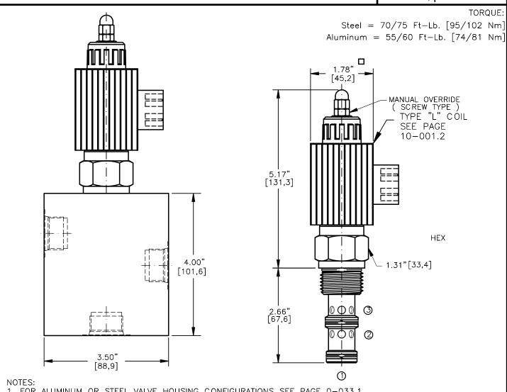
1. FOR ALUMINUM OR STEEL VALVE HOUSING CONFIGURATIONS SEE PAGE 0-033.1 2. SOLENOIDS AVAILABLE WITH DIODES - CONSULT FACTORY.
